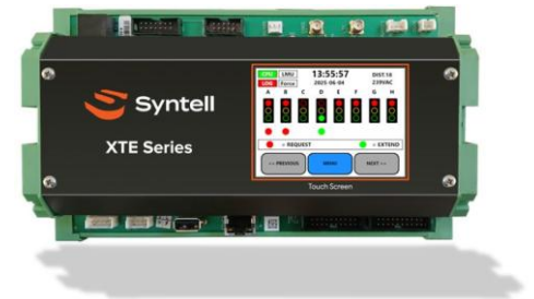
Onboard touchscreen — live module & signal status, no tools required.
